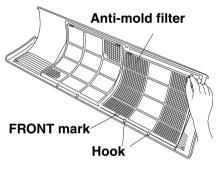
2. Allow the edge of the air intake grille to slide into the top of the indoor unit, and then insert it all the way inside.
