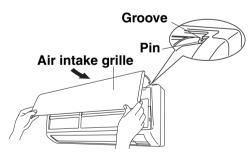
Press in the bottom right and left corners of the air intake grille to attach the indoor unit.
