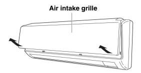
2. Remove the anti-mold filter attached to the rear of the air intake grille.
