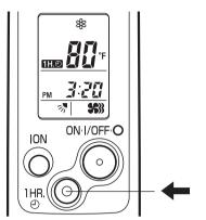
This function causes the unit to operate for one hour and then stop, regardless of whether the unit is on or off when this button is pressed.
