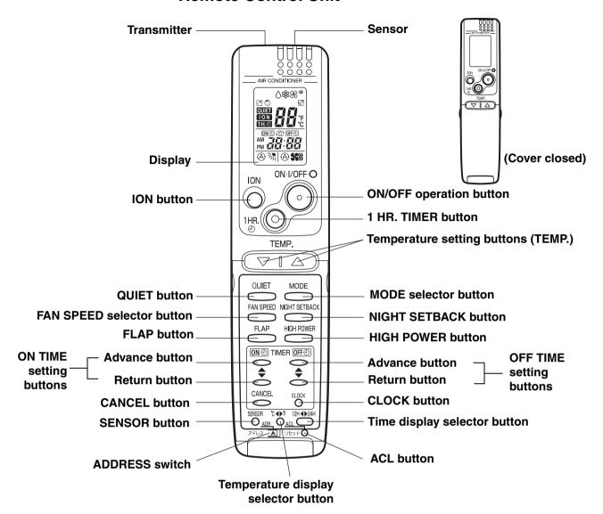
**NOTE** The illustration above pictures the remote control unit after the cover has been opened.
